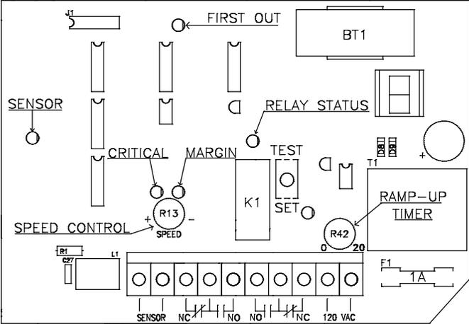
**CRITICAL SPEED LED** - Must be illuminated continuously to allow control relay to energize.
