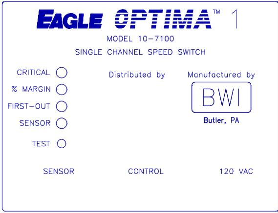
**CRITICAL SPEED LED** - Must be illuminated continuously to allow control relay to energize.
