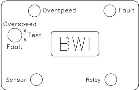
**OVERSPEED LED** - When illuminated, indicates that an overspeed condition was detected by the unit. This is a latching LED that will automatically reset when the Reset input signal has been activated.
