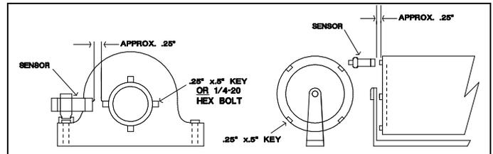
Note: When mounting sensor on small idler rollers (less than 6 inches in diameter), install a maximum of 2 targets
