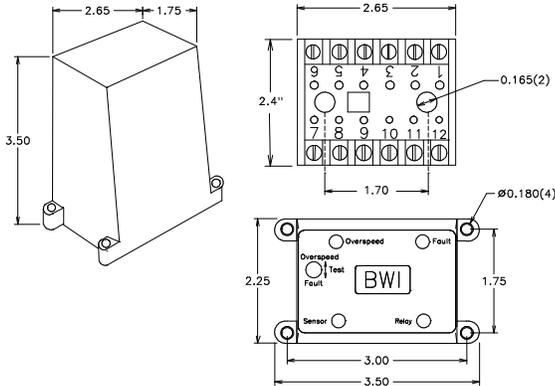
Allow for 5.25" total height with module in socket
