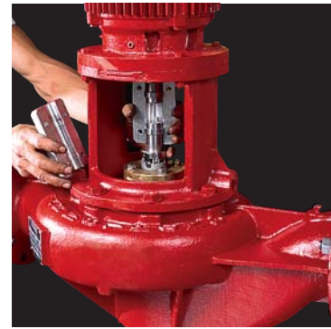
2) Remove the coupling bolts. The coupling halves (with drive and annular positioning keys) are taken from motor and pump shafts. Loosen set screws on seal rotating element and slide from pump shaft. (For inside seal see step 3)
