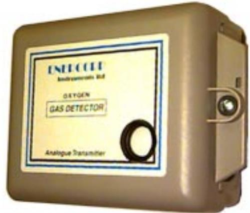
**AST-8000 series** transmitters incorporate wide spectrum solid-state sensors with a life expectancy of 5 years or more. They operate on 24 VDC or 24 VAC input voltages with a 100mA current draw. They are temperature compensated and operate from 0 to 90%rH non-condensing. They are more economical and have a longer life than the AST-7000 series but are less accurate.
