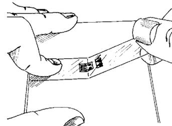
**Note:** Micro-Measurements PCT-2M gage installation tape must be used if tape is employed to position the gage. Other tapes may react with uncured adhesive.
