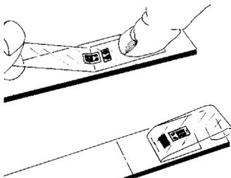
Lift one end of the tape at a shallow angle to surface (about 45 degrees) until gage and terminal are free of specimen surface. Tuck the loose end of the tape under and press to the surface so the gage lies flat with the bonding side exposed. In some cases this may be difficult
