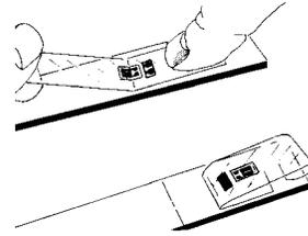
Lift one end of the tape at a shallow angle to surface (about 45 degrees) until gage and terminal are free of specimen surface. Tuck the loose end of the tape under and press to the surface so the gage lies flat with the bonding side exposed. In some cases this may be difficult because of space limitations. If this situation occurs, leave enough slack in the tape to allow a finger to be slipped behind the gage to support it while applying the adhesive.
