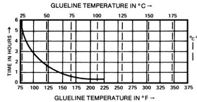
**Caution:** These systems may not cure properly below +70°F [+20°C]. Postcuring the installation for two hours at least +25°F [+15°C] above the maximum operating temperature with the clamping fixture removed will provide essentially creep-free performance.
