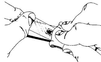
Lift the tuckered-over end of tape and bridge it over the adhesive at approximately a 30-degree angle. With a piece of gauze, slowly make a single wiping stroke over the gage/tape assembly, bringing the gage back down over the alignment marks on the specimen. Use a firm
