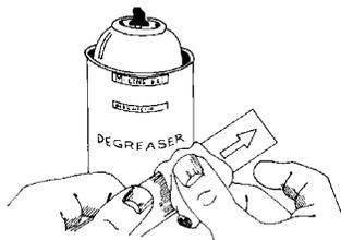
The surface preparation technique used is the same basic cleaning procedure described in Micro-Measurements Application Note B-129, "Surface Preparation for Strain Gage Bonding". The initial step is to thoroughly degrease with solvents such as CSM Degreaser or GC-6 Isopropyl
