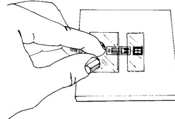
Remove a gage from its mylar envelope with tweezers, making certain not to touch any exposed foil. Place the gage, bonding side down, onto a chemically clean glass plate or empty gage box. If a solder terminal is to be incorporated, position it next to the gage. While holding the gage in position with a mylar envelope, place a short length of MJG-2 mylar tape down over about half of the gage tabs and the entire terminals.
