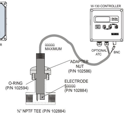
**ELECTRODE HOUSING WITHOUT PREAMP IN-LINE MOUNT**
