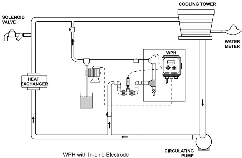
For in-line applications, feed the electrode housing cable through the adapter nut. Remove the protective cap from the end of the electrode cartridge, and thread the cartridge into the housing until it is hand tight. The o-ring should seat against the housing. Place the large o-ring into the mounting adapter groove, then place the electrode housing into the tee, and thread the adapter nut onto the tee until it is hand tight.
