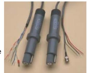
The differential preamplifier and optional automatic temperature compensation (ATC) element are built into the housing, resulting in signal amplification at the optimal location - right next to the sensor. Temperature response is fast, increasing accuracy of measurement.
