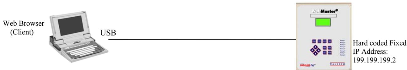
A USB connection to the WebMaster Industrial Water can be made via a temporary cable between a laptop and the front panel of the controller.
