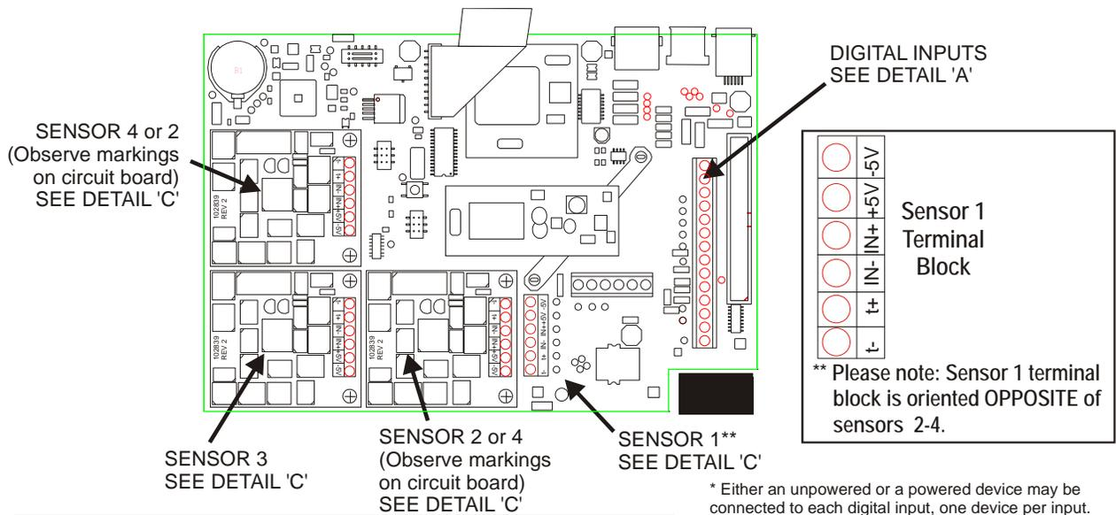
\* Either an unpowered or a powered device may be connected to each digital input, one device per input.
