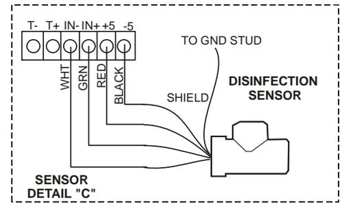
Figure 5: Wiring Diagram for Sensor Inputs and Digital Inputs A-F
