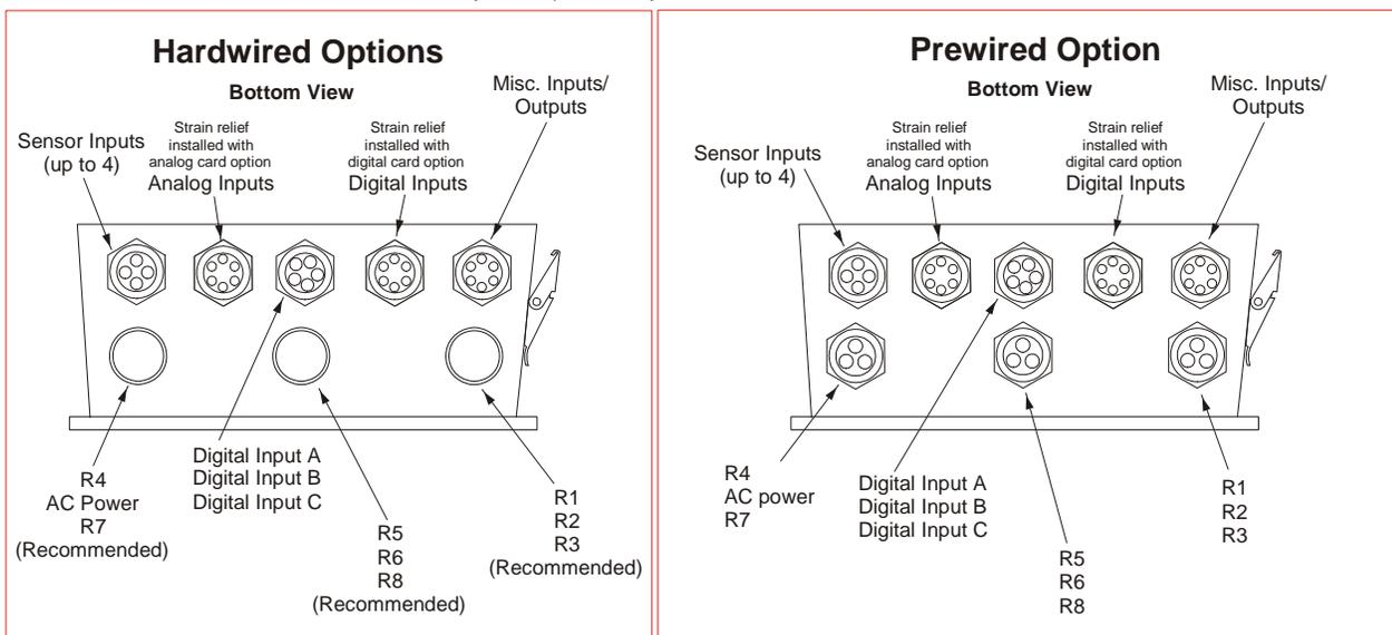
Figure 2: Conduit/Wiring Configuration
