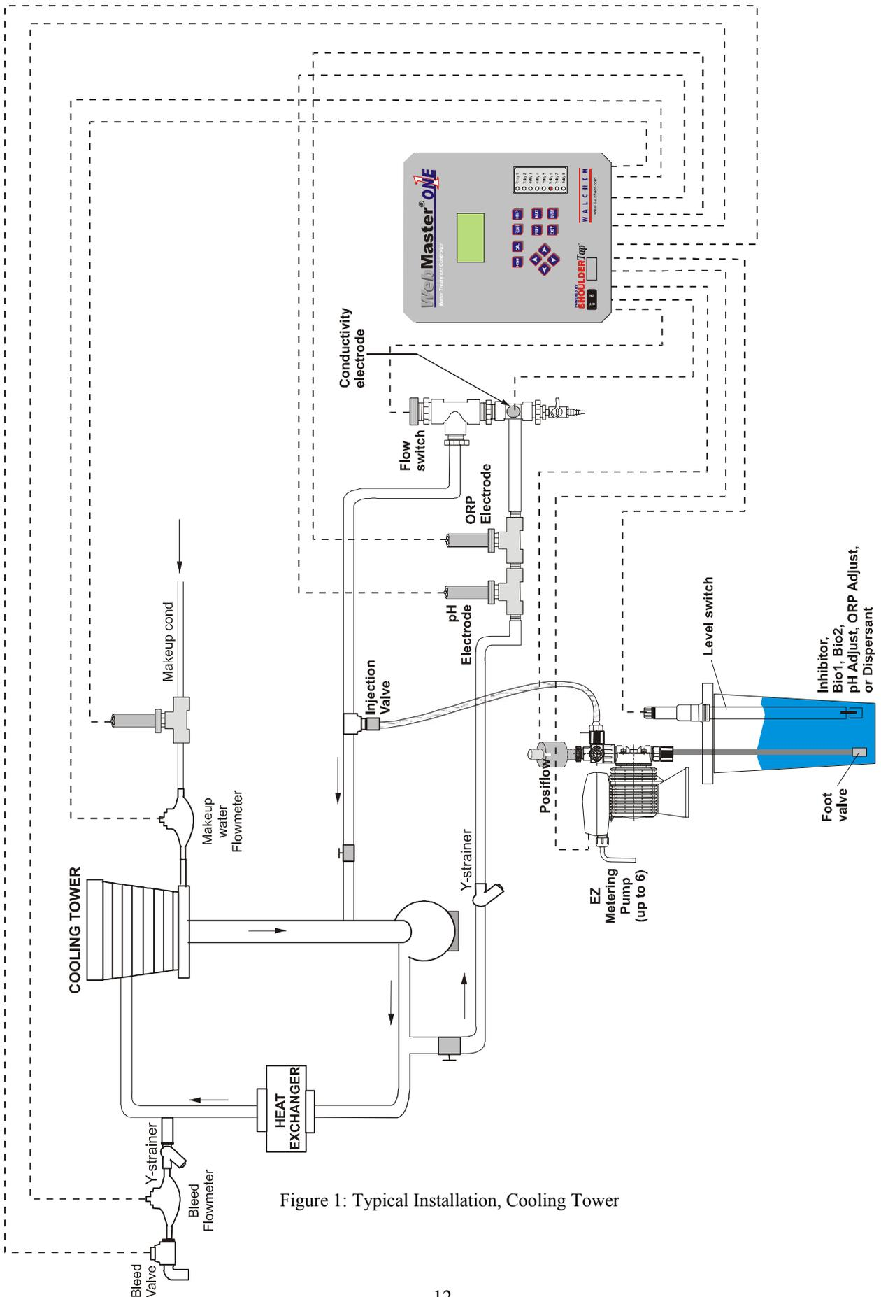
Figure 1: Typical Installation, Cooling Tower
