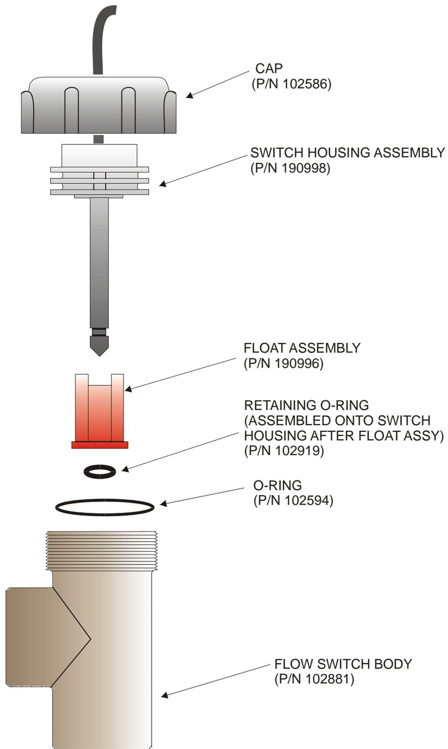
Figure 10 Flow Switch Assembly
