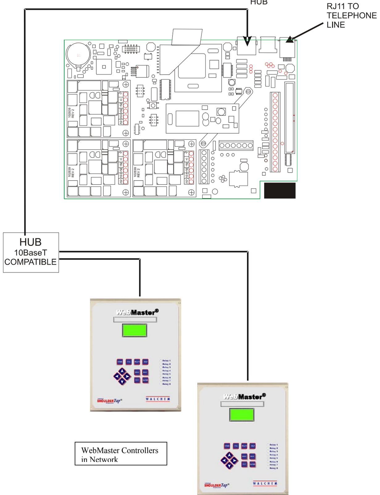
Figure 7: Wiring Diagram for Optional Digital Communications
