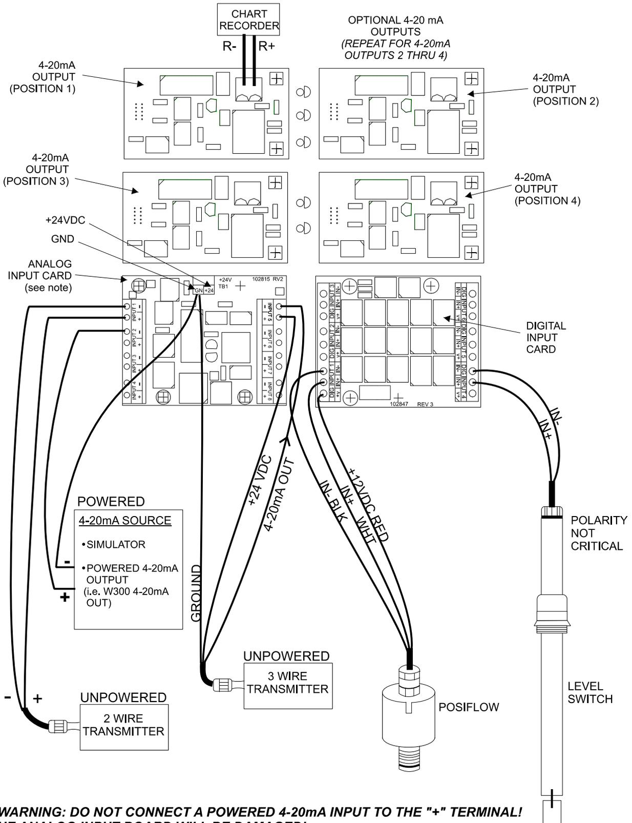
**\* WARNING: DO NOT CONNECT A POWERED 4-20mA INPUT TO THE "+" TERMINAL! THE ANALOG INPUT BOARD WILL BE DAMAGED!**
