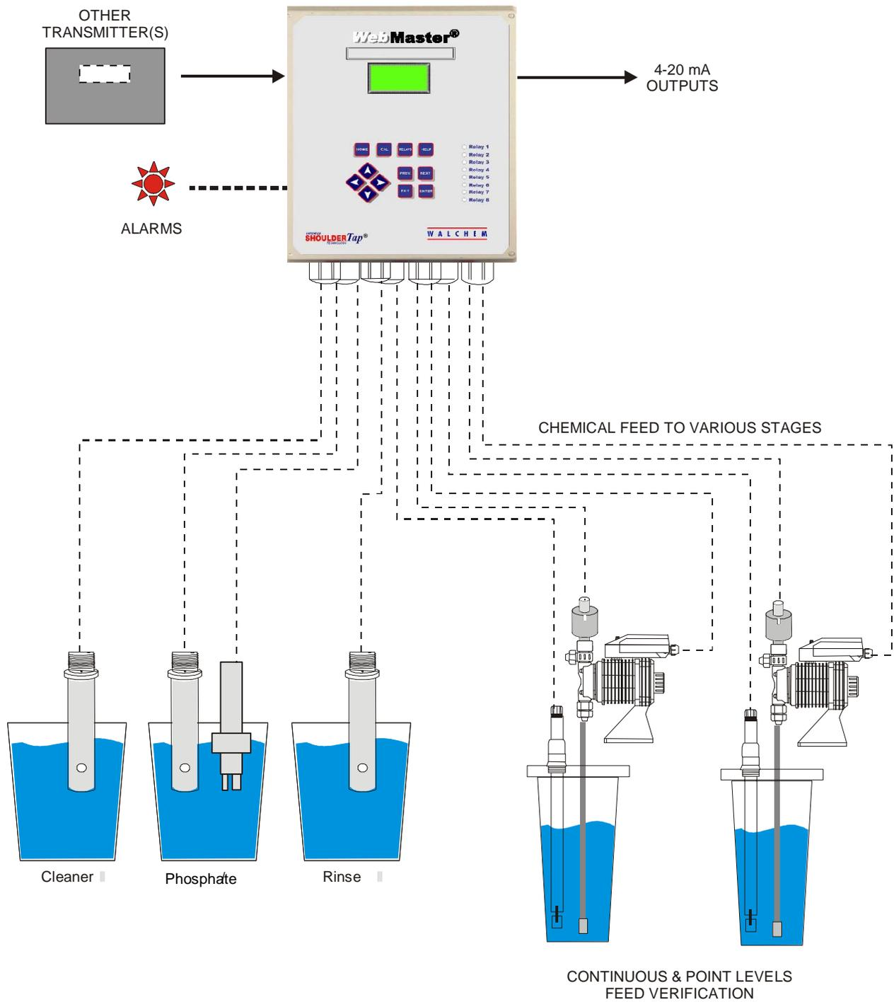
Figure 1: Typical Installation, Parts Washer
