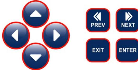
To change a value in a submenu, the left/right arrow keys move the cursor left and right to each digit or option that can be changed. The up/down arrows will change numeric values up or down, or scroll through option choices. Press **ENTER** only when you have finished making all of the changes for that menu screen.
