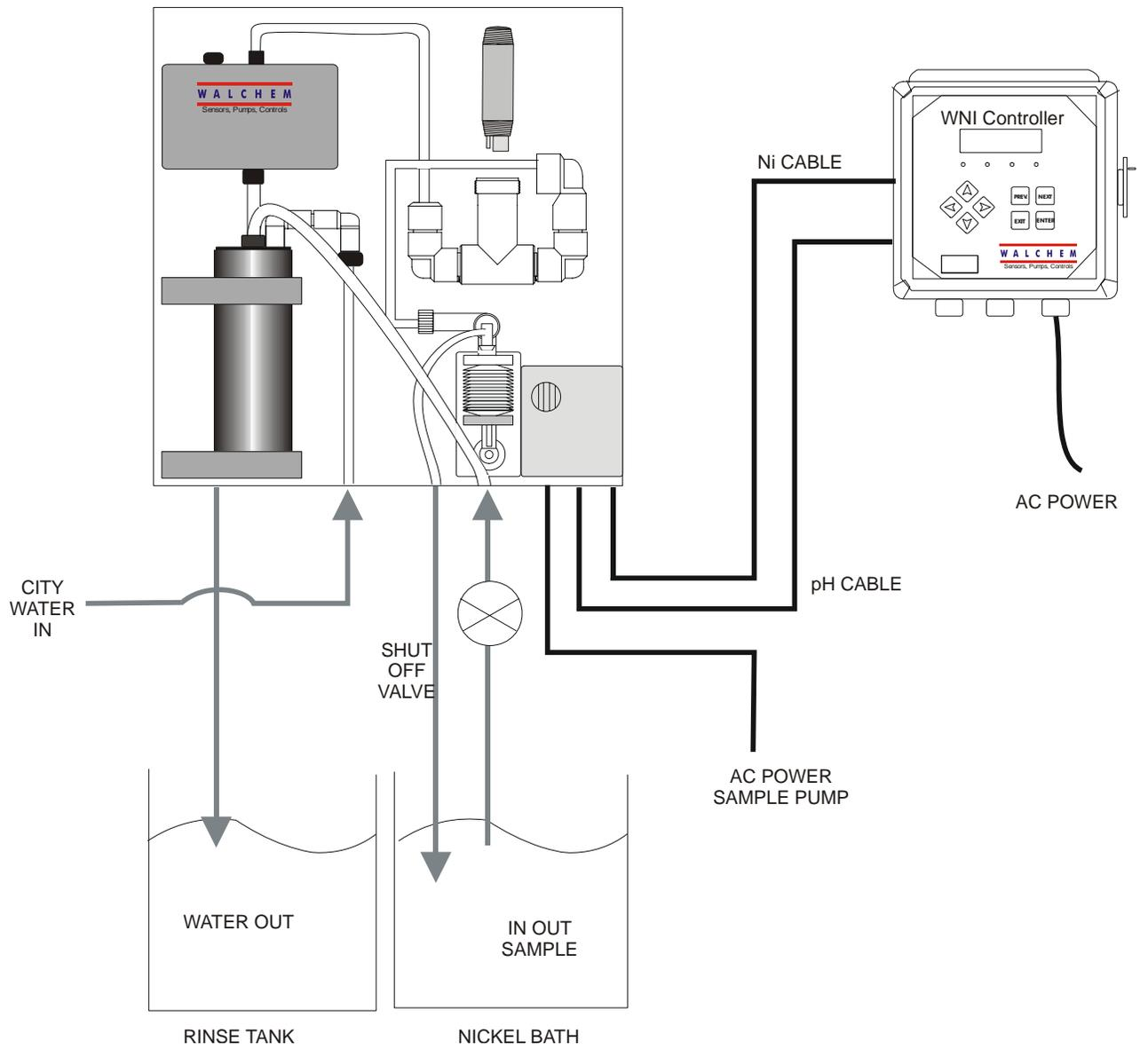
**Figure 1C Electroless Nickel Sample System Installation**
