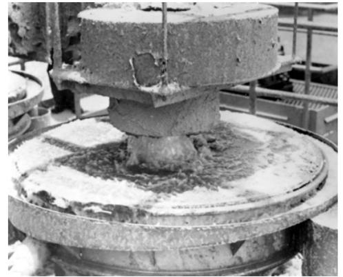
*360° discharge is achieved with Cascade deck design, greatly increasing the capacity of this Kason Separator handling shower water.*
