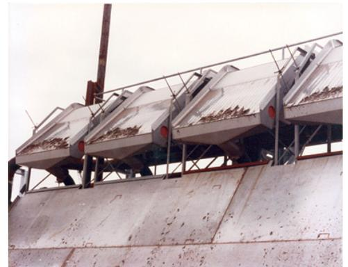
Bank of four Kason "Cross-Flo" sieves screens bark out of the flume water system at once Chesapeake Corporation.
