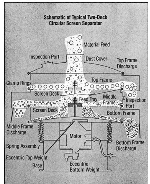
*Schematic of standard 2-deck separator first used in separating polypropylene pellets at the plant*
