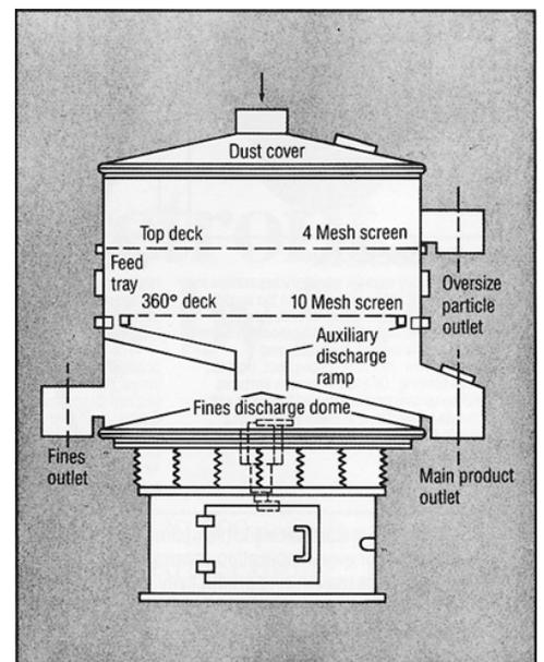
*Schematic of separator retrofitted with high-capacity 360° discharge cone in middle frame and high-capacity inclined discharge ramp with oversized discharge spout in bottom frame*
