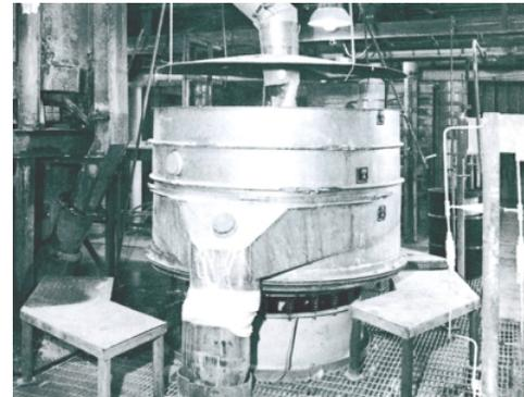
*Retrofitted separator at work in a polypropylene plant. Prime product is discharged from the oversized spout in the foreground*
