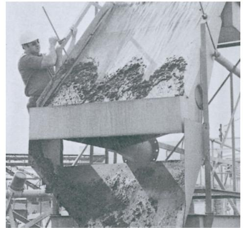
Fig. 2 Operator adjusts the slope of a typical trash-removing Cross-Flo Sieve.
