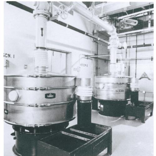
*Two Kason Vibroscreen® units used to collect hair, plastic and other material in the wastewater prior to its transport to a centrifuge for clarification.*
