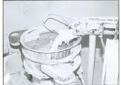
*One of the two stainless steel 48" diameter Kason "Vibro-Screen" separators modified to incorporate a second deck so as to serve as a "Recycled Clarifier" and increase production.*
