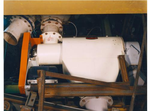
*The centrifugal sifter at the Wilton Armetale foundry removes contaminant materials from casting sand prior to reconditioning and reuses.*
