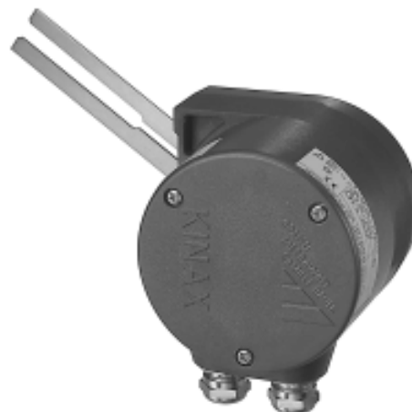
Fig. 2. Position feedback transmitter KINAX SR 709 showing the operating lever in the upper zero position, corresponding output current 0/4 mA.
